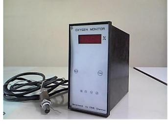
measuring the oxygen percentage in stack gas monitoring (upto  $350^{\circ}$ C) which in turn gives combustion efficiency of oil-fired boilers. It is used in oil fired boilers to monitor the combustion efficiency & CO emission and can also be used to monitor the stack gas (temperature below  $350^{\circ}$ C).
